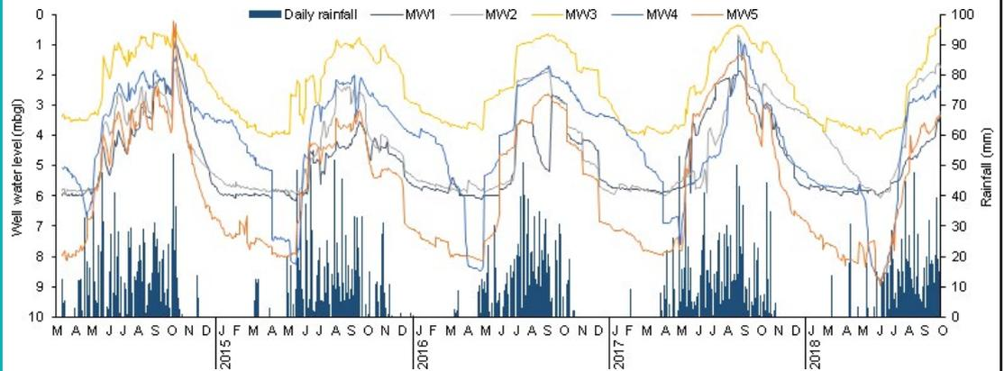
FIGURE B3: Plot showing daily rainfall and groundwater level in five monitoring wells (MW) from the Dangila CBM.
