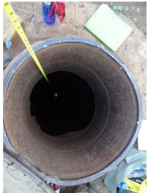
FIGURE 12. (a) and (b) Measuring groundwater levels in hand-dug wells in Boloso Bombe *woreda*. Photos from: David Walker.
