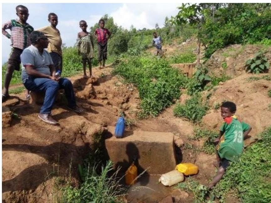
FIGURE 13. Measuring spring flow in Boloso Bombe *woreda* utilising a jerry can and mobile phone stopwatch. Photo from: David Walker.
