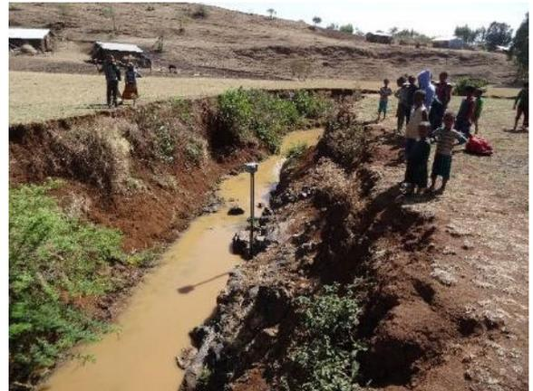
FIGURE 4. (a) A tipping-bucket automatic rain gauge installed in Dangila *woreda* in an open, level area beside the observer's house; note the protective fence. (b) A river staff gauge secured to bedrock in Dangila *woreda* (this particular staff gauge includes a pressure transducer for automatically monitoring river stage; the box on the top of the gauge contains a datalogger). Photos from: David Walker.
