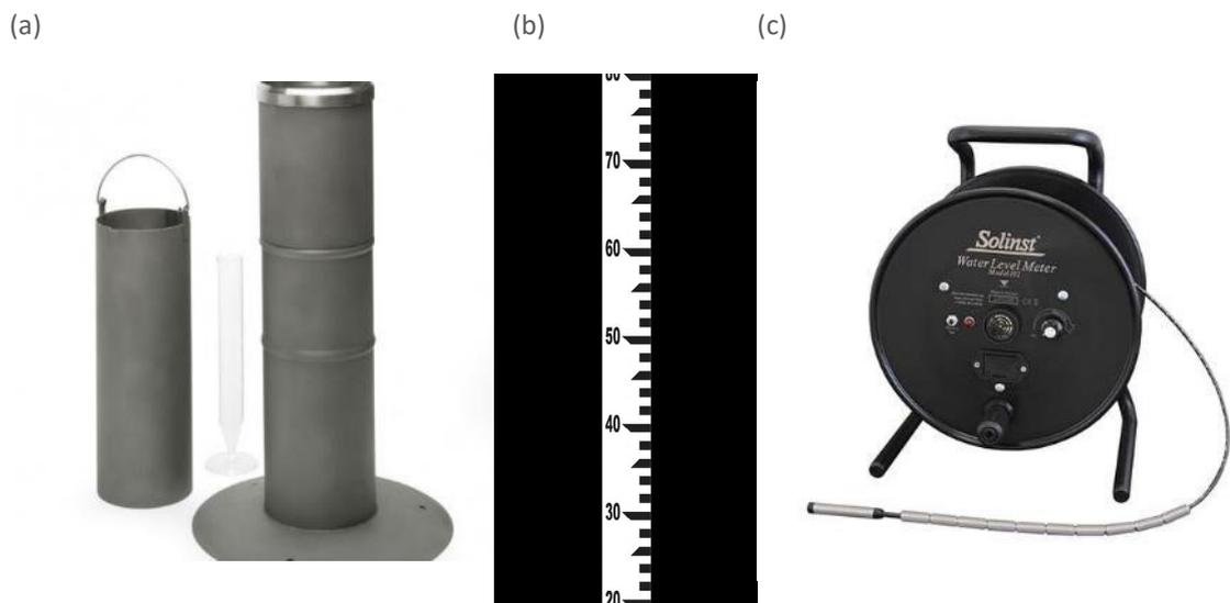
FIGURE 2. Typical CBM equipment: (a) manual rain gauge, (b) staff gauge, (c) dip-meter.
