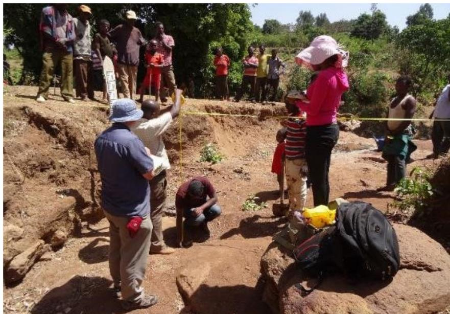
FIGURE 9. Surveying the channel profile at a newly installed river staff gauge in Boloso Bombe *woreda*. Photo from: David Walker.
