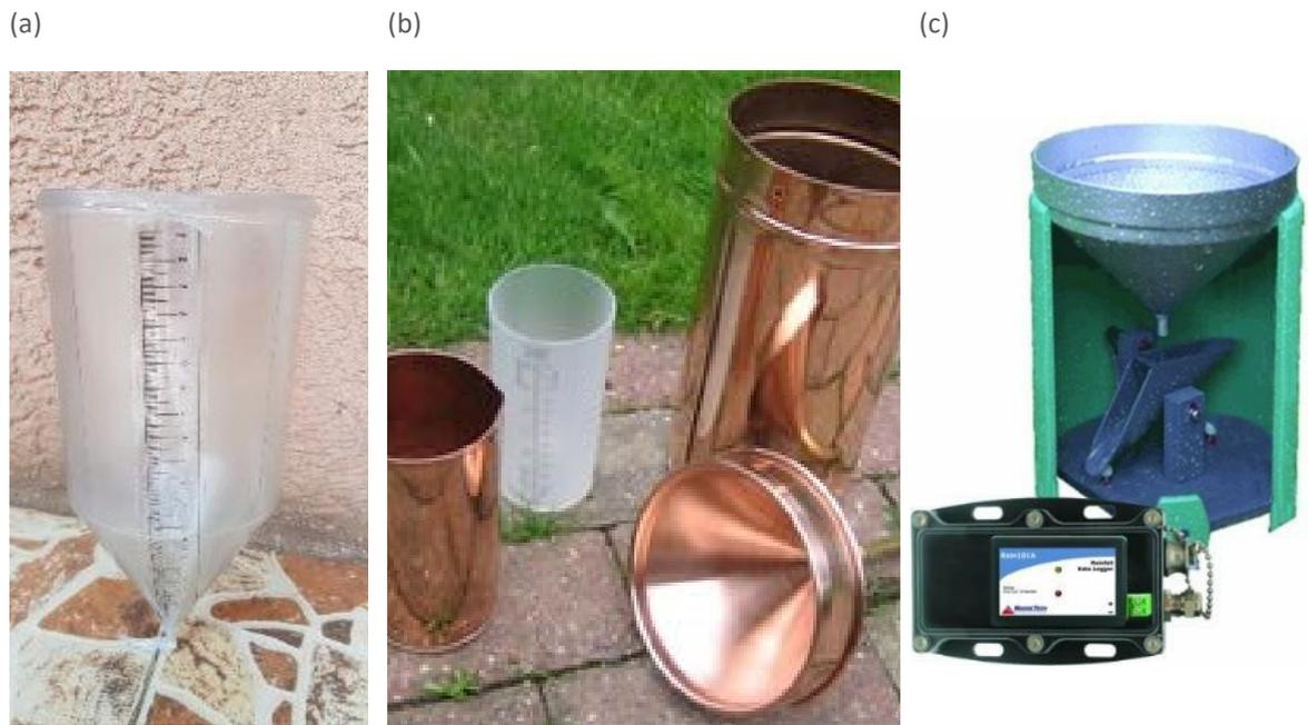
FIGURE 6. Different types of rain gauge: (a) a low-cost plastic manual gauge, (b) an expensive copper manual gauge (this is a design recognised by international standards for rainfall monitoring), and (c) a tipping-bucket automatic gauge. Photos from: Mintamer Ferede.
